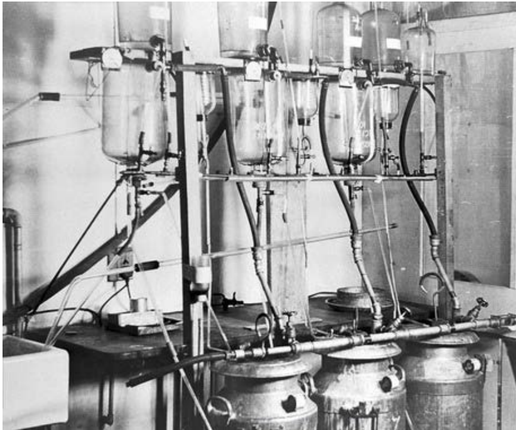
Glass flasks and milk churns used for making early forms of penicillin
